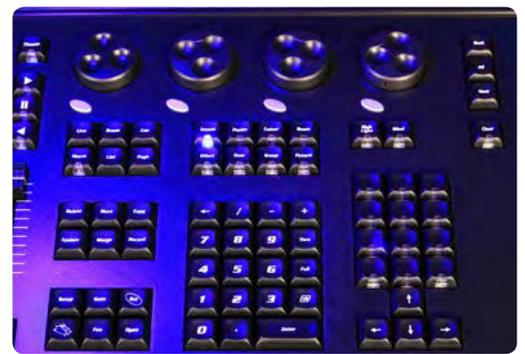
The four encoders have small clear/silver buttons adjacent and these allow you to do a variety of things such as jumping values. Much of the console can be customized including the bank of function keys, which can do anything from selecting fixtures through to playing cue lists. Assigning cue lists to faders initially confused me a little, but it's just a case of different button sequencing from what I expected. Once you get that through your head it's all good.
